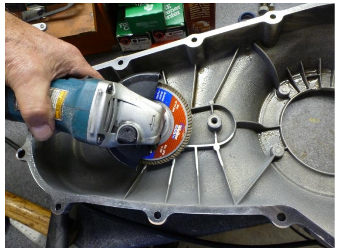
Figure 6; Clearancing with a angle grinder
