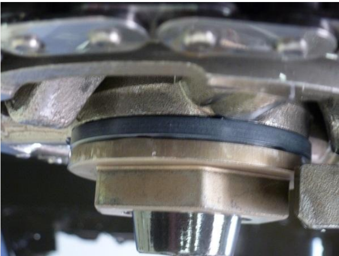
Figure 8; Composite thrust washer installed
