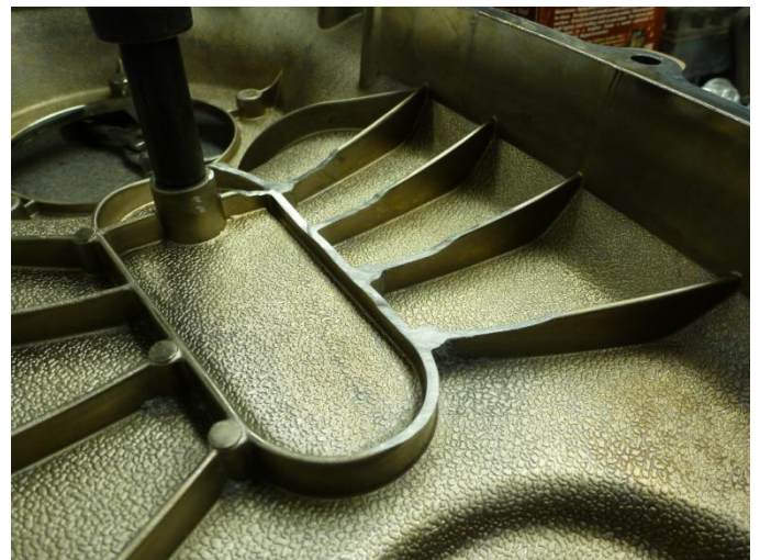
Figure 5; Softtail model rib removal for oil tray
