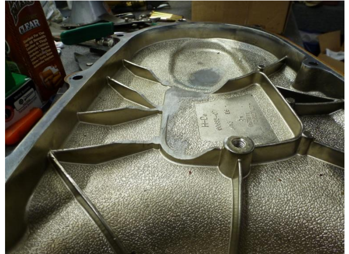
Figure 4; touring model rib removal for oil tray
