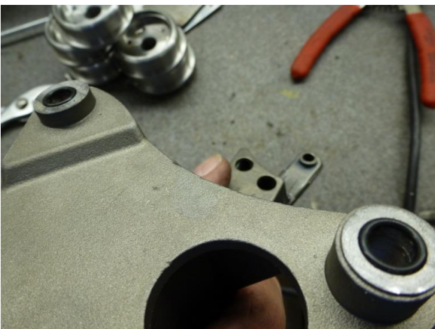
Figure 3: Placement of O-Rings
