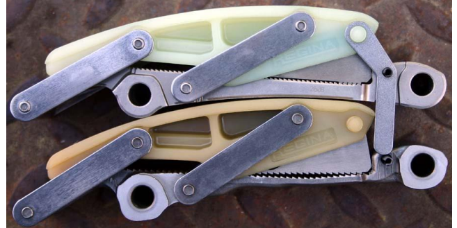
Figure 10; Harley Auto chain adjuster 07+models years 39929-06B is the latest version
