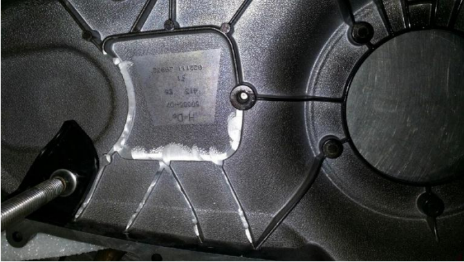
Figure 7; installing the SE oil scoop is necessary on retrofit applications where the scoop is not cast into the cover
