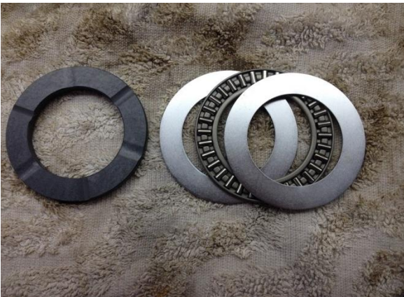
Figure 9; Composite washer to be installed. The 3 part axial roller thrust bearing to be discarded.
